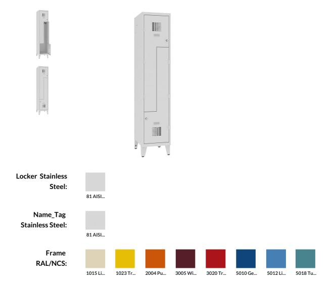
Wardrobe locker locked with 1-point cylinder locks. Each compartment equipped with a bar with 2 hooks and a self-adhesive name plate. Door with registered industrial design of modern look. Doors with enhancement made of 0.6 mm thick steel, other elements made of 0.5 mm thick steel. Wardrobe locker with L-shaped doors. Equipped with 140 mm high lev ...
